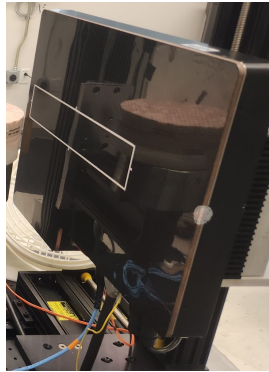
2D planner 30 x 5cm 2 CdTe based detector with 100 µm pixel size (Xcounter)
