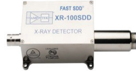
1 pixel 5x5x1 mm 3 Silicon based detector (Amptek)
